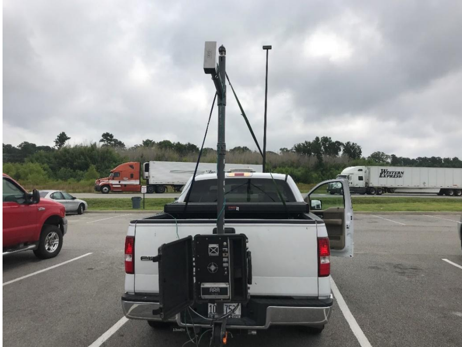
Figure 2: PaVision server unit with downward camera and GPS antenna above
