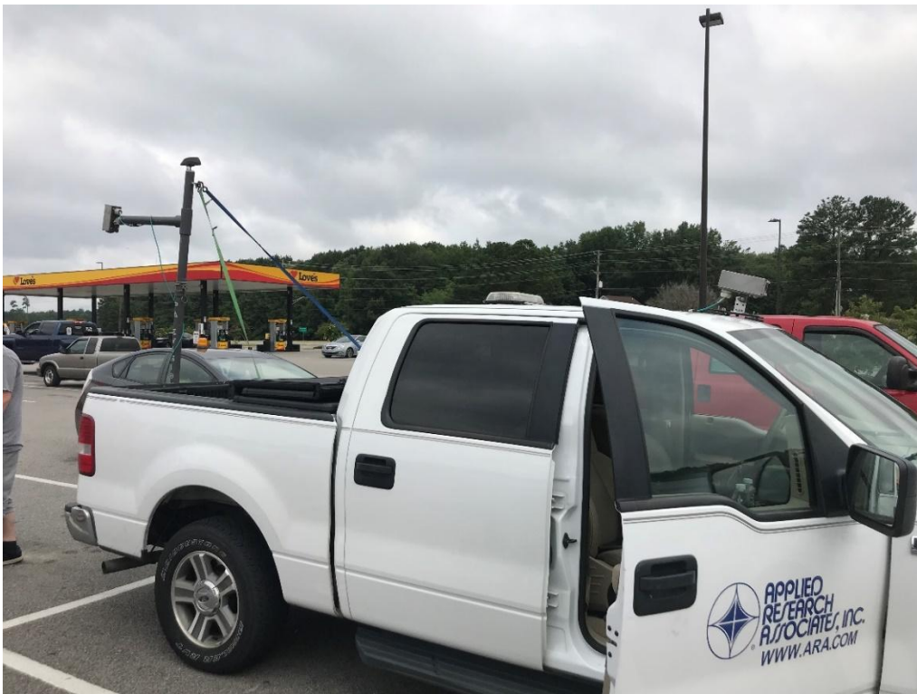
Figure 1: ARA vehicle with PaVision unit on the hitch and forward camera above windshield
